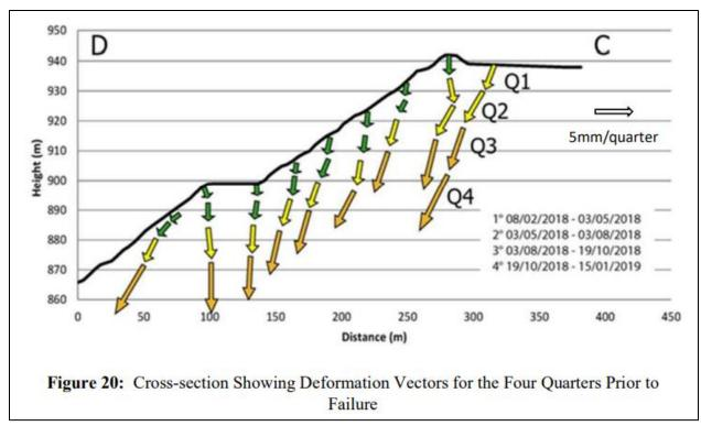
**Figure A11.** The downward creep of tailings due to gravity in the year preceding the failure of the Brumadinho tailings dam caused an increase in the shear stress on the iron oxide bonds between the tailings (see Figs. A10a-b). Because of the brittle nature of the iron oxide bonds, a small strain caused a large increase in shear stress (see Fig. A12). Figure from Robertson et al. (2019).
