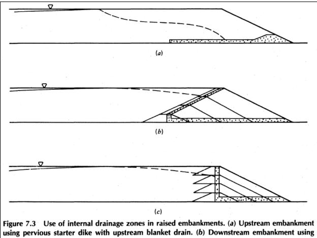
using pervious starter dike with upstream blanket drain. (b) Downstream embankment using inclined chimney drain and blanket drain. (c) Centerline embankment with vertical chimney drain and blanket drain.
