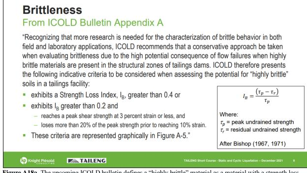
**Figure A18a.** The upcoming ICOLD bulletin defines a "highly brittle" material as a material with a strength loss index greater than 0.4. Slide from Ridlen (2021).
