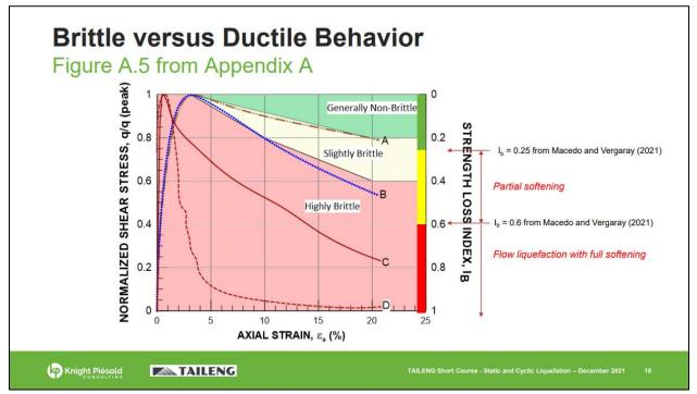
**Figure A18b.** The upcoming ICOLD bulletin defines a "highly brittle" material as a material with a strength loss index ( $I_B$ ) greater than 0.4 (see Fig. A18a). According to Macedo and Vergeray (2021), "The trends suggest that flow liquefaction cases with partial softening may have in general a  $I_B$  larger than 0.25 ... whereas the flow liquefaction cases with full softening may be associated with  $I_B$  values higher than 0.6." Slide from Ridlen (2021).
