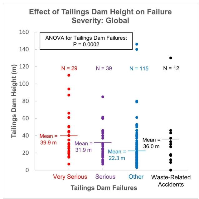
**Figure A28a.** For global failed tailings dams (including failed tailings dams in the USA), the differences among the mean heights of dams that underwent Very Serious (39.9 meters), Serious (31.9 meters feet) and Other (22.3 meters) Tailings Dam Failures are statistically significant at better than the 99.9% confidence level (P = 0.0002). Wasterelated Accidents were not included in calculations of P-values. Data and severity codes from Center for Science in Public Participation (2022):
