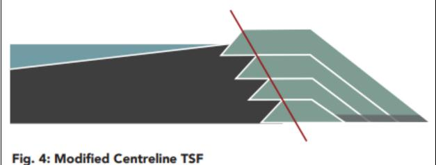
**Figure 8.** Although Centerra Gold (2022) claims that the tailings dam at the Kemess South facility (with a height of 180 meters) was constructed using the "modified centerline" method, the construction is actually a variation on the upstream method, since the dikes are constructed on top of the uncompacted tailings (compare with Figs. A2a and A2c). In fact, ICOLD (2021) refers to the construction method as "modified upstream" (see Fig. A22). Figure from Centerra Gold (2022).
