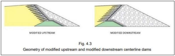
**Figure A22.** The above diagram from ICOLD (2021) confirms that what has been called the "modified centerline" method (see Fig. A21) should be referred to as the "modified upstream" method. The so-called "modified centerline" method retains the essential characteristics of the upstream method in that successive dikes are constructed on top of uncompacted tailings (compare with Fig. A2a). Figure from ICOLD (2021).
