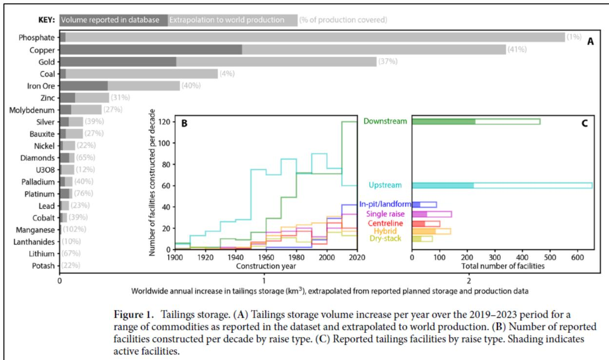
**Figure 1.** Tailings storage. (A) Tailings storage volume increase per year over the 2019–2023 period for a range of commodities as reported in the dataset and extrapolated to world production. (B) Number of reported facilities constructed per decade by raise type. (C) Reported tailings facilities by raise type. Shading indicates active facilities.
