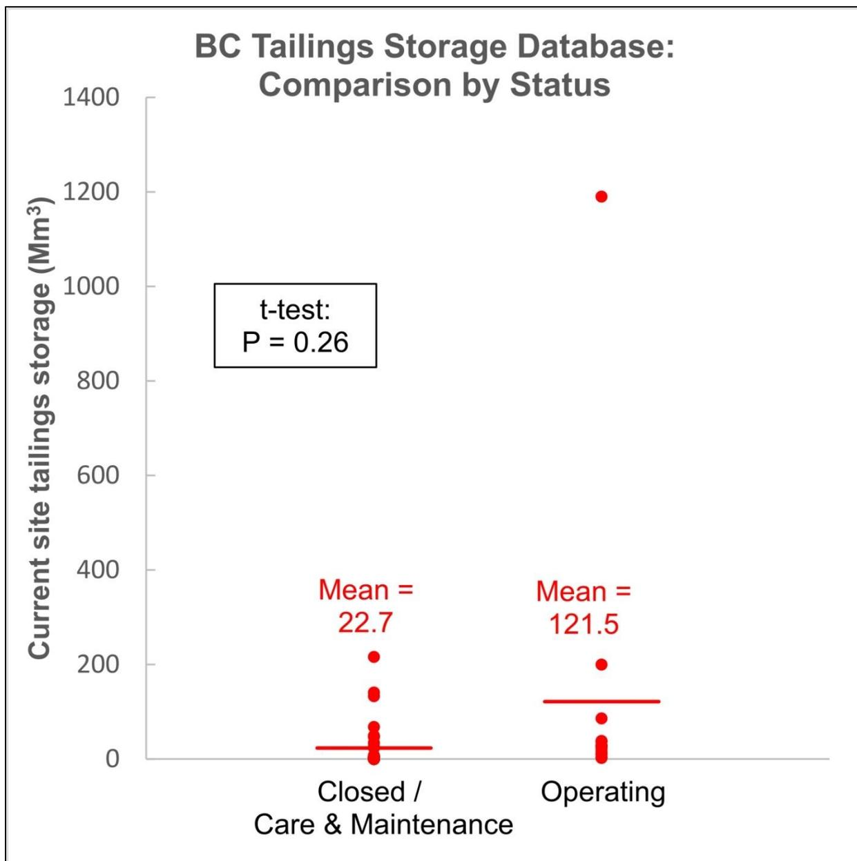
**Figure 2b.** For the BC Tailings Storage Database, the site-wide tailings storage volumes were compared between the 57 sites that are closed or under care and maintenance and the 18 operating sites. According to the t-test, the difference between the mean site storage at the sites that are closed or under care and maintenance (22.7 million cubic meters) and the operating sites (121.5 million cubic meters) is not statistically significant ( $P = 0.26$ ).
