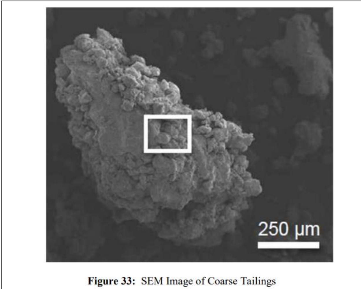
**Figure A10a.** The high iron oxide content of the iron-ore tailings at the Brumadinho tailings storage facility promoted the dissolution and re-precipitation of iron oxides and, thus, the formation of iron oxide bonds between the tailings. See close-up of iron oxide bonding in Fig. A10b. Figure from Robertson et al. (2019).
