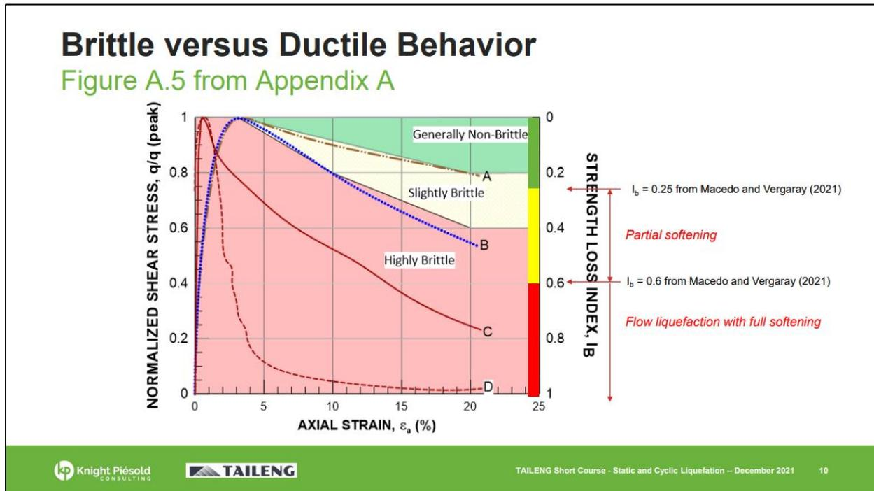
**Figure A18b.** The upcoming ICOLD bulletin defines a “highly brittle” material as a material with a strength loss index ( $I_B$ ) greater than 0.4 (see Fig. A18a). According to Macedo and Vergeray (2021), “The trends suggest that flow liquefaction cases with partial softening may have in general a  $I_B$  larger than 0.25 ... whereas the flow liquefaction cases with full softening may be associated with  $I_B$  values higher than 0.6.” Slide from Ridlen (2021).
