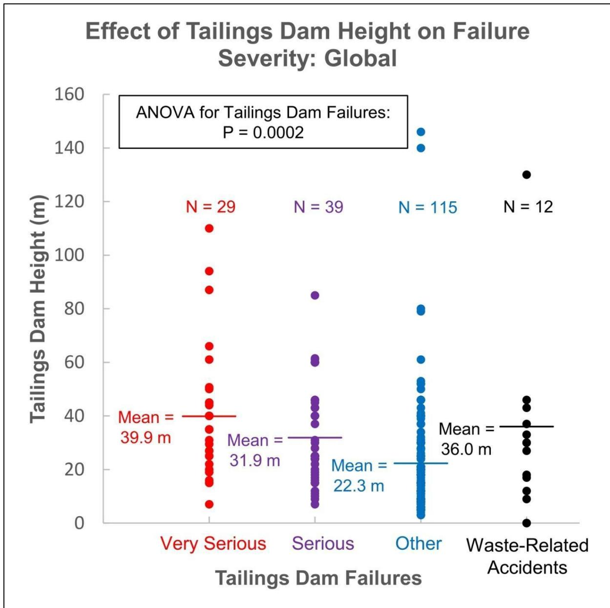
**Figure A28a.** For global failed tailings dams (including failed tailings dams in the USA), the differences among the mean heights of dams that underwent Very Serious (39.9 meters), Serious (31.9 meters) and Other (22.3 meters) Tailings Dam Failures are statistically significant at better than the 99.9% confidence level ( $P = 0.0002$ ). Waste-related Accidents were not included in calculations of P-values. Data and severity codes from Center for Science in Public Participation (2022):
