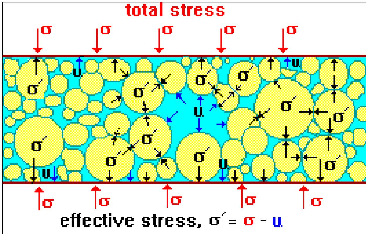
**Figure A3.** The effective stress in soil is equal to the total stress minus the pore water pressure. The effective stress is a measure of the extent to which the solid particles are interacting with or “touching” each other. Terzaghi’s Principle states that the response of a soil mass to a change in stress is due exclusively to the change in effective stress. Figure from GeotechniCAL (2022).
